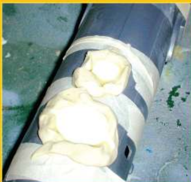
Small 'dams' of modelling clay were built around the turret openings to prevent the resin from flowing all over the model.
