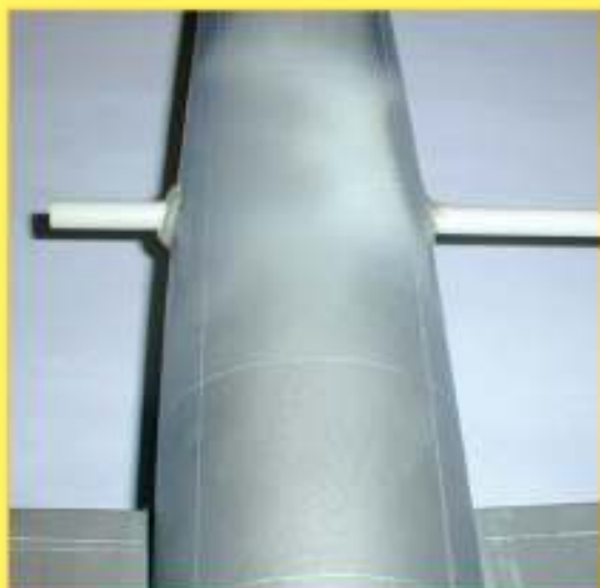
Plastic tube used to resize the small fuselage windows as explained in the text.
