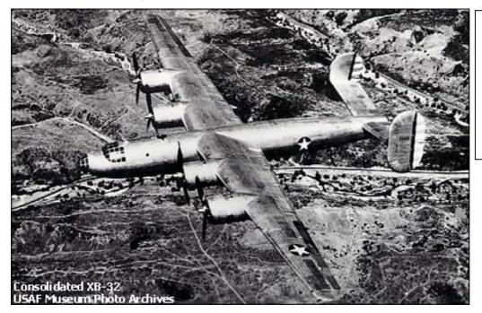
The second XB-32 (41-142). Note the twin tails and fully glazed nose – both of which would disappear before the B-32 got into production. (USAF Museum)
