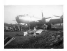
Above: Loading the spare engine into the bomb bay of the
