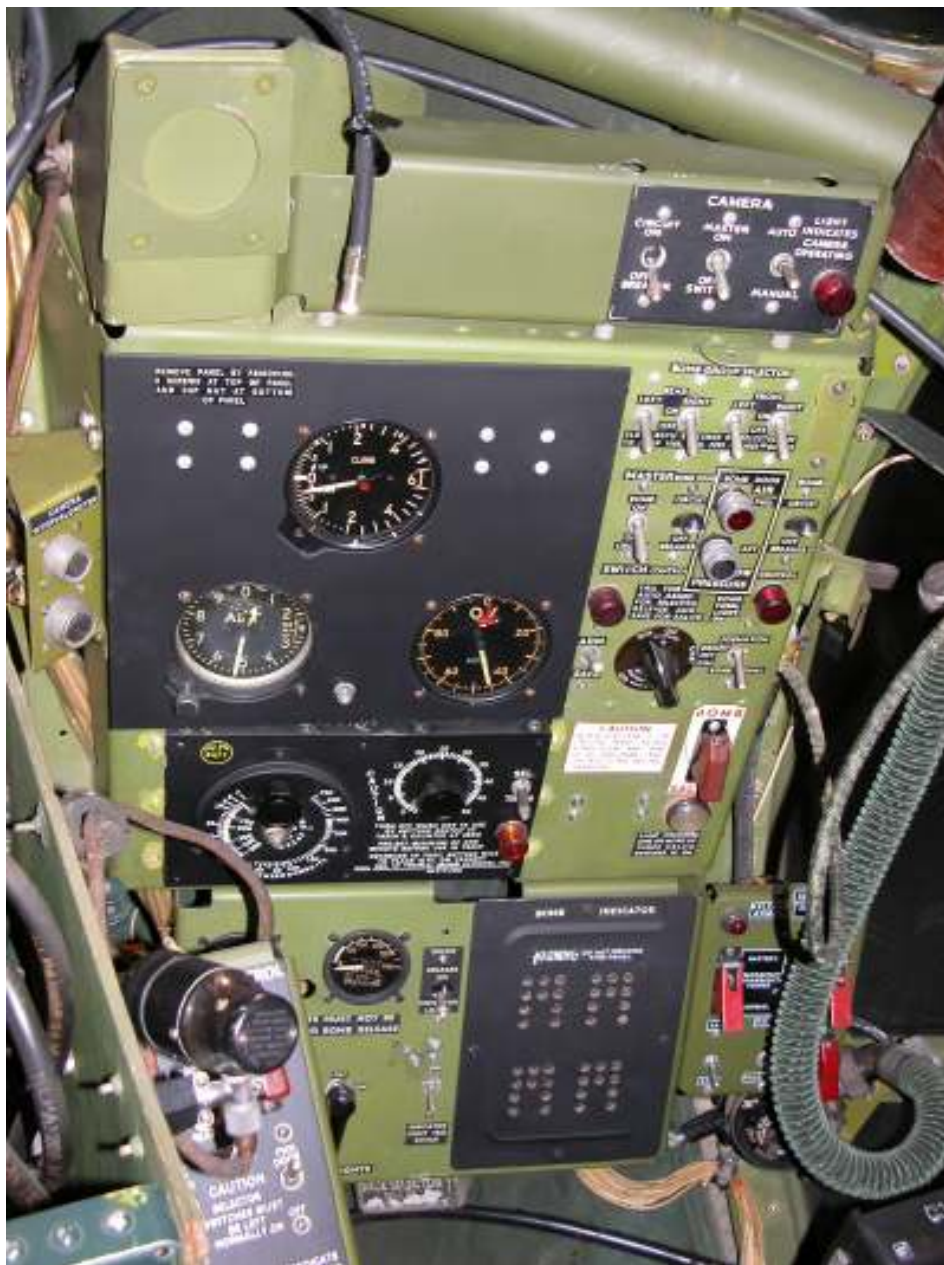
Bottom: The 'High Altitude Absolute Altimeter' (SCR-718) in Enola Gay . (Bernie Poppert)
