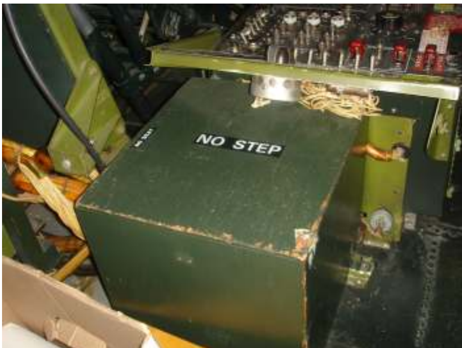
Left: The protective plywood box covering the vertical flight gyro located just behind the central aisle stand in Enola Gay . ( Taigh Ramey )
