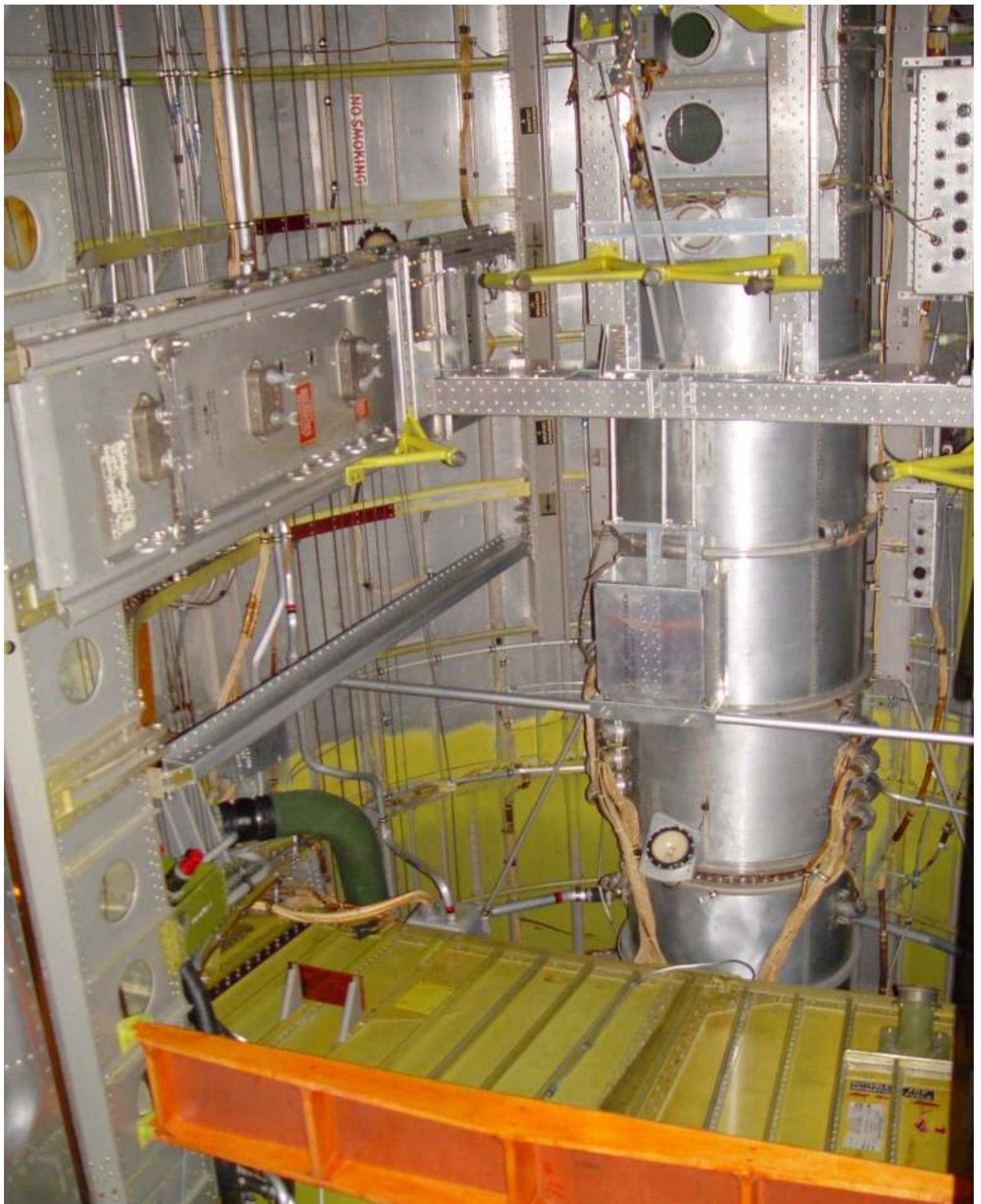
Above: Looking up into the forward bomb bay ( Mike Hanz ). Note the communication tunnel running along the top of the bomb bay. The raised section of the communication tunnel with its viewing window can be seen above the bomb suspension (extreme top of photo). Either side of the window are two additional ports that allowed limited access to the shackle should this be required. The yellow/green box is the wing centre section. Immediately behind this, above the catwalks in the rear bomb bay are the gear boxes that allowed the main landing gears to be raised or lowered in an emergency. The gear box on the right hand side operated the let hand gear. The gear was moved via a hand crank and required some 774 turns to raise (about 30 minutes of effort) or 387 turns to lower (about 12 minutes of effort).
