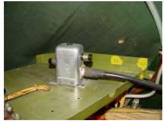
Above: The signal splitter on the shelf above the Radio Operator's station in Enola Gay ( Mike Hanz )
