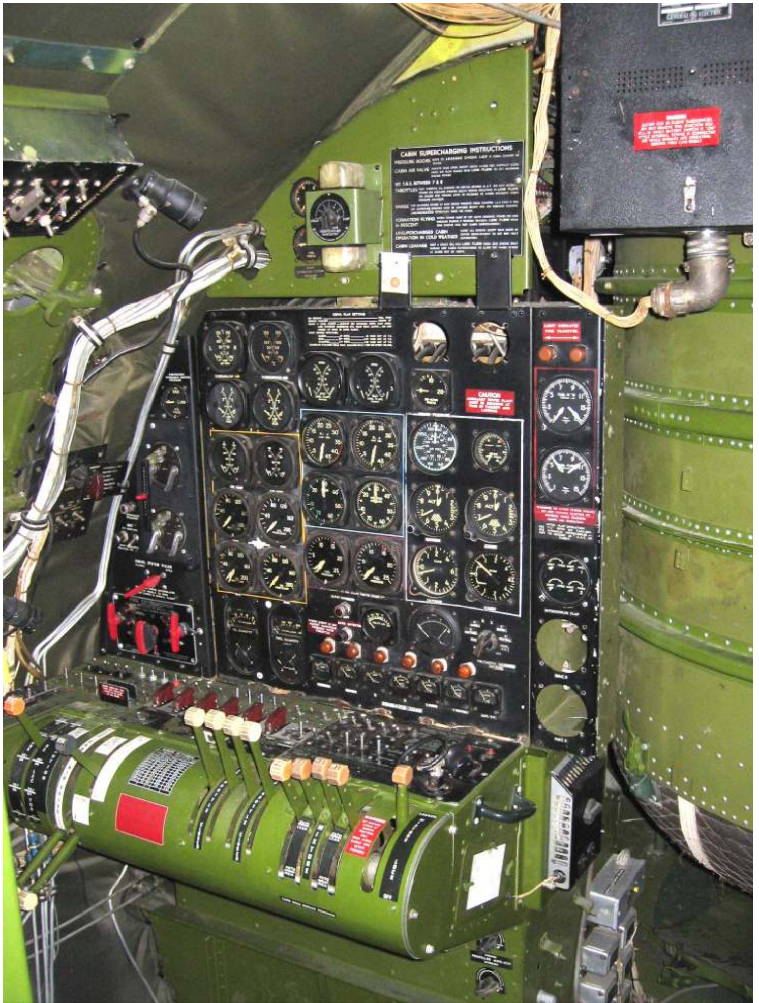
Above: The Flight Engineer's station in It's Hawg Wild – a B-29A fitted with the Transfer Fuel system. ( Ivor Warne ) Note the black box connected to the front of the upper forward gun turret tub. This is the servo amplifier for the lower forward gun turret. The servo amplifier for the upper forward gun turret is located in the rear gunner's compartment (see page 59).
