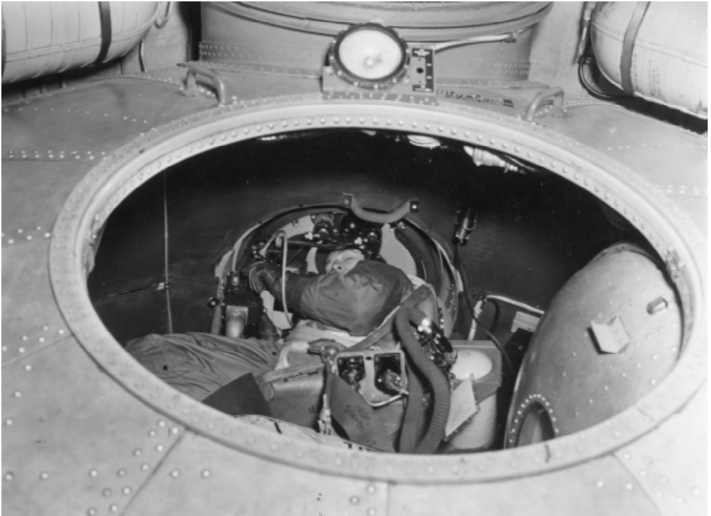
**Left:** Photographed from the rear bomb bay through the hatch in the bulkhead a CFC gunner occupies the Barber's Chair. (*PRB1698*)
