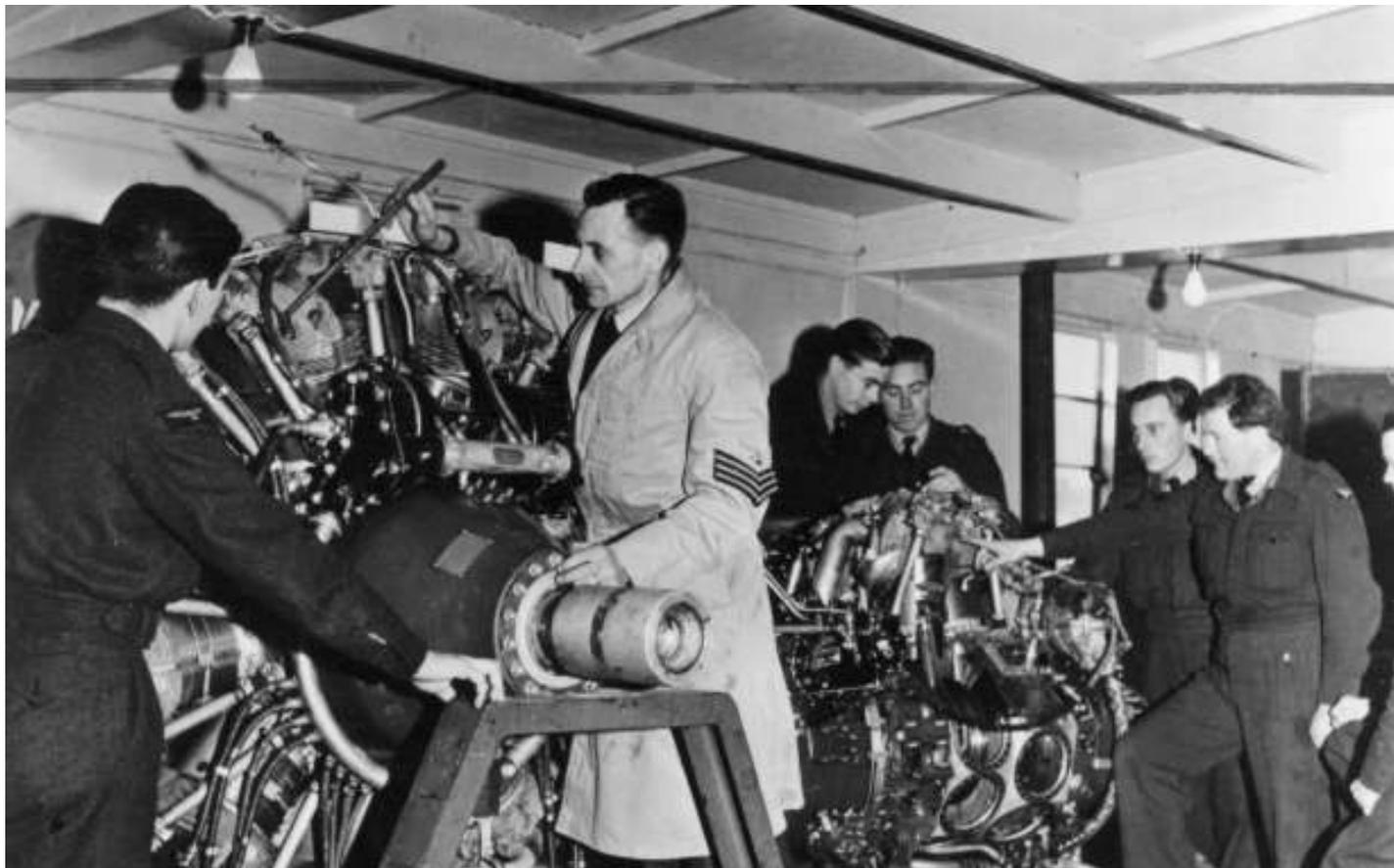
**Above:** Newly trained Engine Fitters get instruction on the mighty Wright R-3350 Duplex Cyclone. RAF engine fitters were generally trained on the Bristol Hercules sleeve valve engine and some conversion training was necessary before they could be let loose on squadron aircraft. (*PRB1669*)
