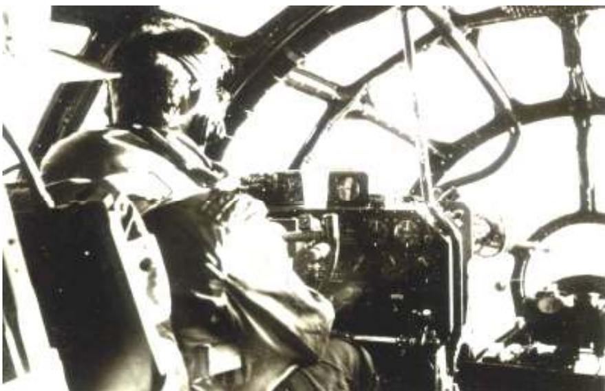
Another interesting piece of equipment on the central console is the Honeywell-Minneapolis autopilot. There are a bunch of 'dash pots' and adjusting knobs that go with this very reliable gadget. Serviceability is its second name and it seldom packs up, unlike the dreadful abominations that appeared in the Lanc and Lincoln. Tie it into the bomb sight during a bomb run and it's money for old rope.
