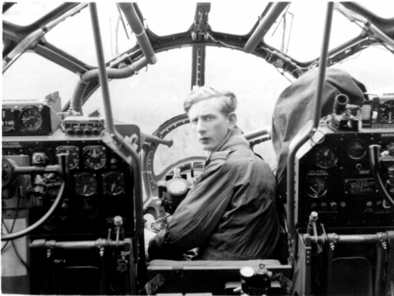
**Above:** Not a clear shot but the best I have of a Norden bomb sight in a Washington. 44 Squadron Nav/Bomb Aimer Gordon Galletly occupying the bomb aimer station. Note the X-1 reflex sight addition to the bomb sight head. Note also the covered forward gun sight and partial views of the Airplane Commander's and Co-pilot's instrument panels. (*Gordon Galletly*)
