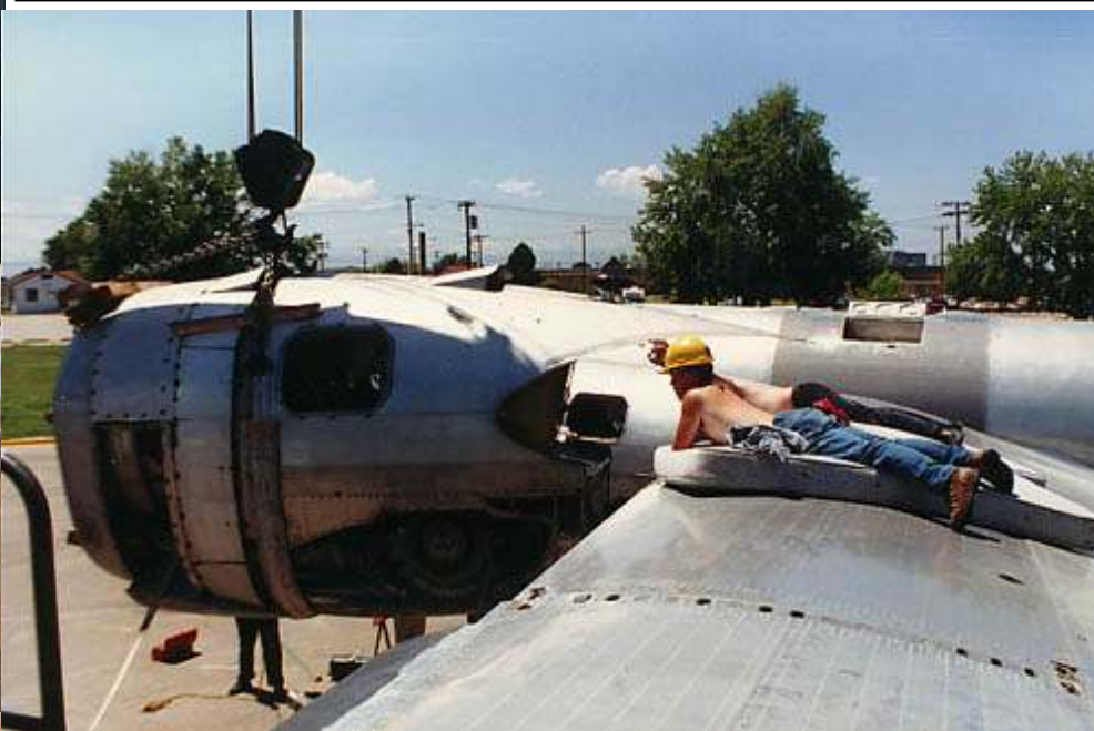
Clockwise from top left: Number 1 engine being re-fitted. Ensuring the engine aligns correctly (note the mattress – the exposed metal became very hot in the sun and would burn bare flesh!). Working on a propeller. Propeller Hub made from old fire extinguishers. Refitting the nose wheels. Fairing in the dummy lower rear gun turret. The original, and several longerons, had been removed during #729's conversion to a tanker. Working on the horizontal stabilizer. (All photos T Sq 54 web site)
