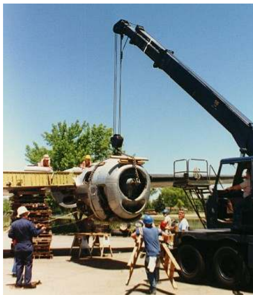
Clockwise from top left: Number 1 engine being re-fitted. Ensuring the engine aligns correctly (note the mattress – the exposed metal became very hot in the sun and would burn bare flesh!). Working on a propeller. Propeller Hub made from old fire extinguishers. Refitting the nose wheels. Fairing in the dummy lower rear gun turret. The original, and several longerons, had been removed during #729's conversion to a tanker. Working on the horizontal stabilizer. (All photos T Sq 54 web site)
