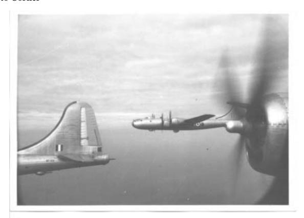
149 Squadron in close formation. Note streamlined turret on plane in distance. This makes it WF547, one of the 2 RAF B-29s with such a turret. Note also the erased '8'(?) on WF491's tail, presumably a remnant of its US service. (*Jeff Brown*)
