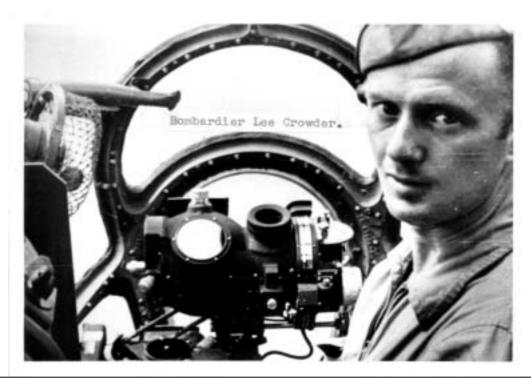
Keeping with the bomb aimer theme, a fine view of the Norden bombsight, this time in a USAAF B-29 on Guam during WWII. Lee Crowder, the bombardier and photographer was taking a serious risk in taking this photo. The Norden was a classified piece of equipment and if discovered the photo would have earned Lee a sever punishment! (*Lee Crowder* via *Jeff Brown*)
